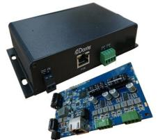
85W @4Ω bridged or 42W x 2ch @8Ω \* CEA-2006, THD+N=1% with external 56V DC input
